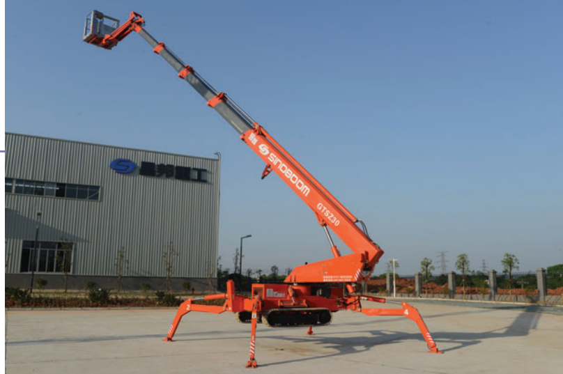
Products on Sinoboom's stand will include the GTSZ30 spider lift, which can reach up to 30 m and boasts a wireless remote control device that works up to 100 m away.
