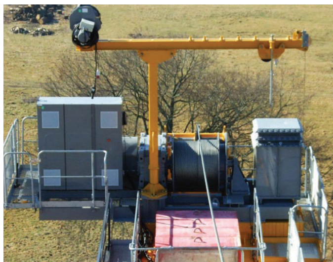
Potain's latest winch is the 270 LVF, a 200 kW machine that can handle loads of up to 40 tonnes in four falls at a maximum speed of 162 m/min.
