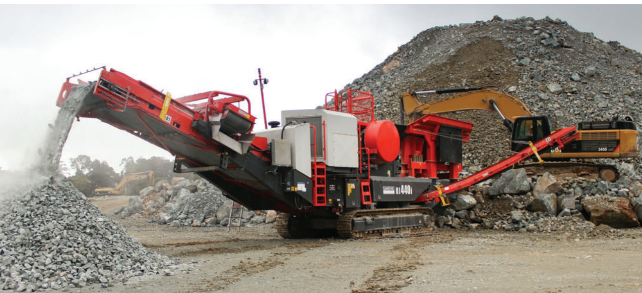
This Sandvik UJ440i mobile crusher is used to produce aggregates from a unique site in Panama which is also a gold mine.
